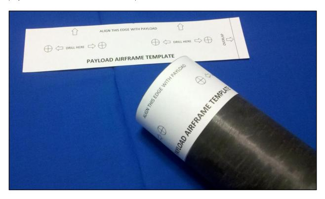
Use the drill and one of the rocket cradles to carefully drill the four holes marked on the drill template. The drill should pass through both the airframe and the nosecone coupler. Once the holes are drilled, the nosecone will most likely only line up one way with the airframe holes.
