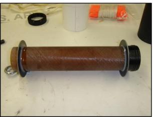
Spread some epoxy on the outside of one end of the motor tube and slide the ring (without the hole) until there is approximately 1/2" of motor tube exposed. Make sure the motor tube is cleaned of any epoxy so as not to interfere with the fin tangs later. After the aft ring is dry, Spread some epoxy on the motor tube and slide the forward ring until it aligns with the mark. Set aside and allow epoxy to harden for at least 10 minutes.
