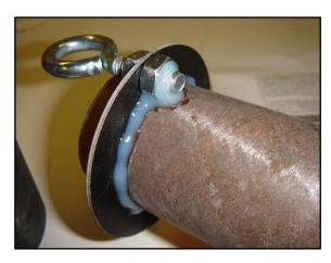
**VERY IMPORTANT**: Make sure there is not any epoxy on the motor tube that would interfere with the fin tangs later on. Make sure there is not any epoxy in the motor tube that would interfere with the motor case later on.
