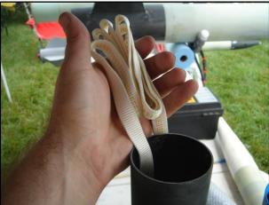
Loosely wrap the folded parachute into the parachute protector. The parachute folding directions are in the recovery section of this workbook. Place the parachute inside of the rocket with the stitched loop facing the top.
