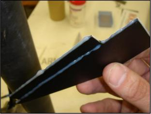
Continue rechecking the fin alignment until it is certain the epoxy has set. Clean any excess epoxy from around the fin joint. Repeat for the remaining fins. Next, apply epoxy fillets to both sides of each fin by applying a thin bead of epoxy at the fin-body tube joining. Carefully smooth the epoxy fillets with your finger before the epoxy sets. Allow each fillet to set before rotating the airframe for the next fillet.
