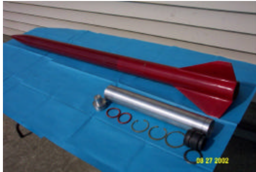
Pictured: Walt's scratch built 3" minimal diameter rocket with experimental 3" L motor casing and internal components.
