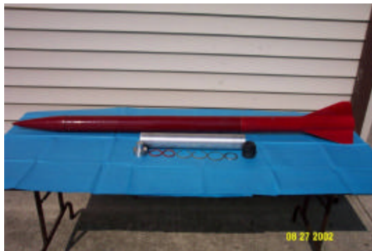
Pictured: Walt's scratch built 3" minimal diameter rocket with experimental 3" L motor casing and internal components.
