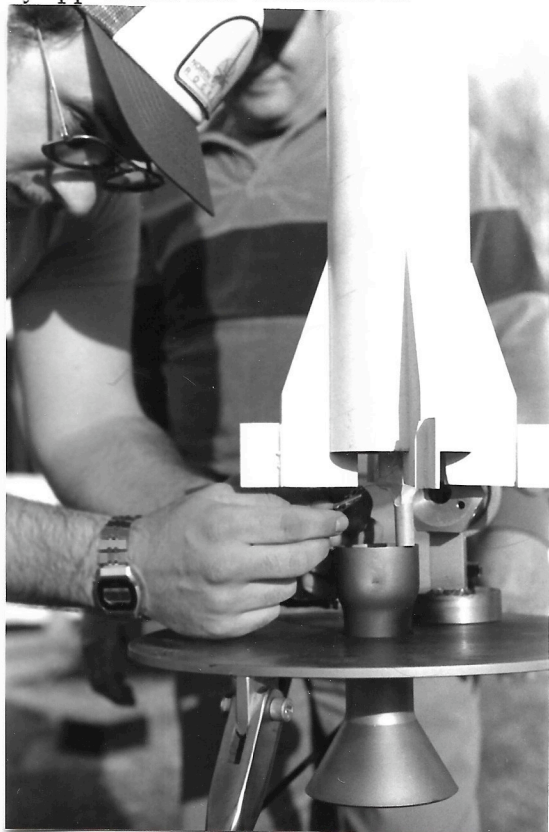
Matt hooks up the 'G' motor to the boilerplate Juno-1 model. The jet deflector in this launcher belonging to Jimmy Williams is from a military rocket nozzle.
